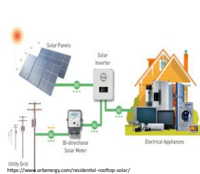
Grid-connected rooftop solar systems
