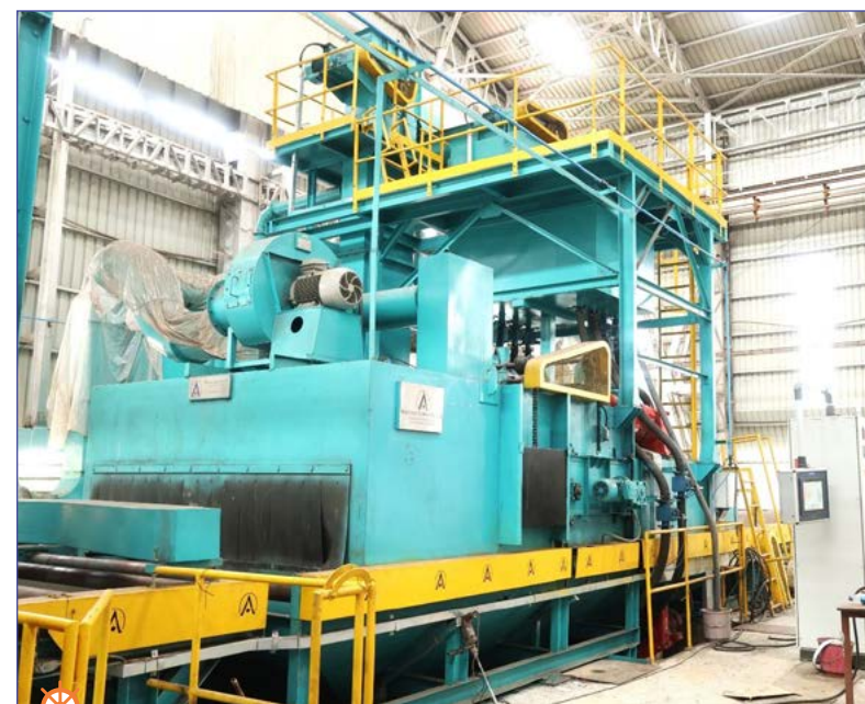
Shot Blasting and Priming Plant
