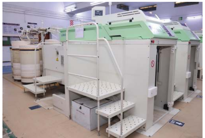
A view of new "LMW-LDB3" Draw Frame Machine installed in our Unit at Rajapalayam.
